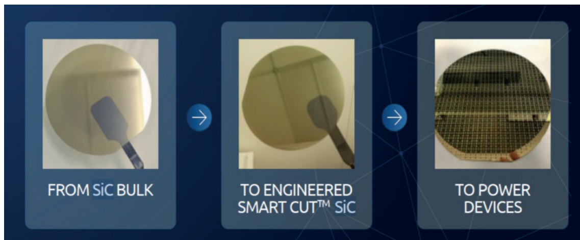
► Figure 3. Pictures of bulk SiC (left), Smart Cut SiC (centre), and Smart Cut SiC with devices (right).
