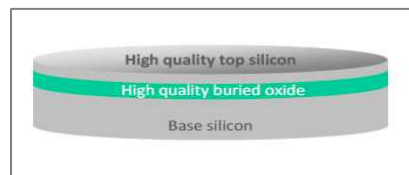
Fig. 3: general structure of a silicon-on-insulator wafer
