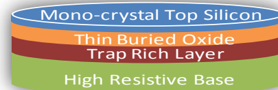
Figure 7: Soitec Wave SOI eSI wafer
